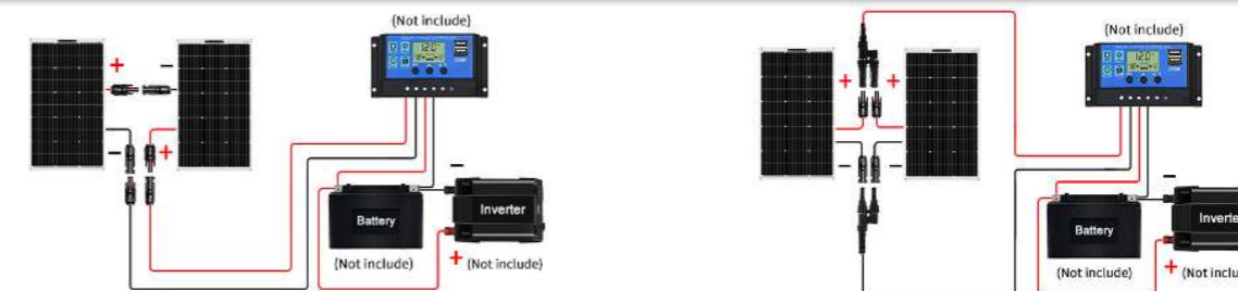
How to connect in series
